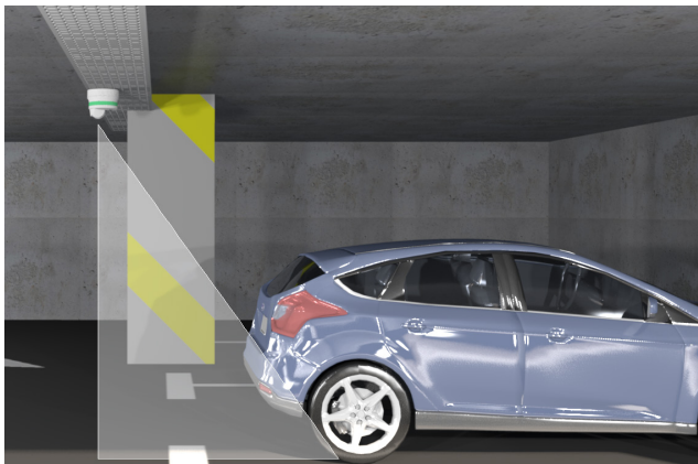
The SBPBASEA is wrongly mounted on the left hand of the cable tray
