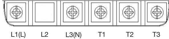
Note: the screw on L2 terminal is removed for the single phase input supply models
