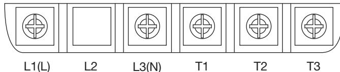
Note: the screw on L2 terminal is removed for the single phase input supply models
