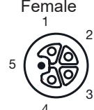
Female M12 connector pinout diagram showing 5 pins: 1 (US+) at top, 2 (UA-) at middle-left, 3 (US-) at middle-right, 4 (UA+) at bottom-left, and 5 (functional earth) at bottom-right. |
