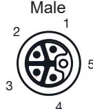
Male M12 connector pinout diagram showing 5 pins: 1 (US+) at top, 2 (UA-) at middle-left, 3 (US-) at middle-right, 4 (UA+) at bottom-right, and 5 (functional earth) at bottom-left.   |
